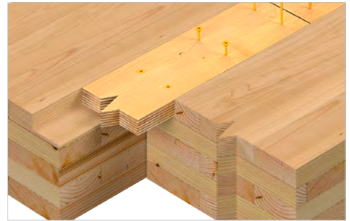
SWC screw installed in a CLT spline.
