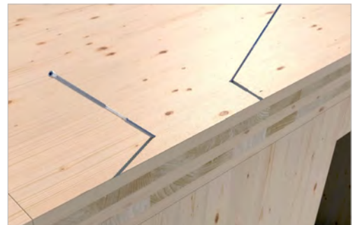
SWD inclined installation of CLT floor panels.
