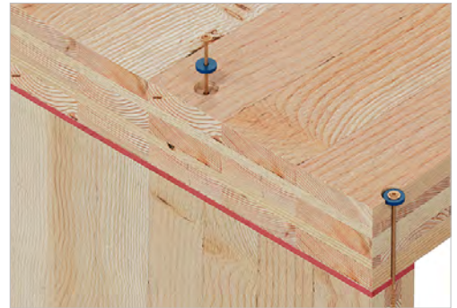
SWW screw installed in a sound insulated CLT floor application.
